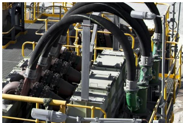
Figure 11. Pumping facility for injecting concentrate
