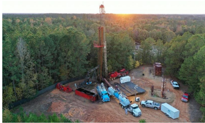
Figure 14. Direct well mining of lithium in The Smackover Formation deposit, Arkansas, US, which is a limestone aquifer with a high concentration of lithium
