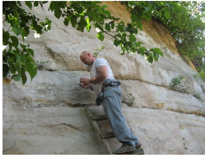
Figure 4. Measurement of elements of the inclination of strata - western slope. (Photo A. Čomić, 2011)
