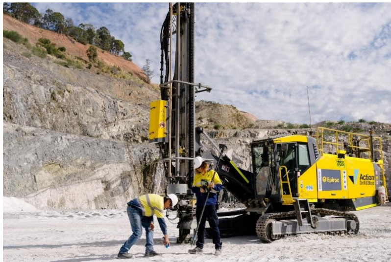
Figure 3. Drilled blastholes at Talison Lithium's Greenbushes in Australia
