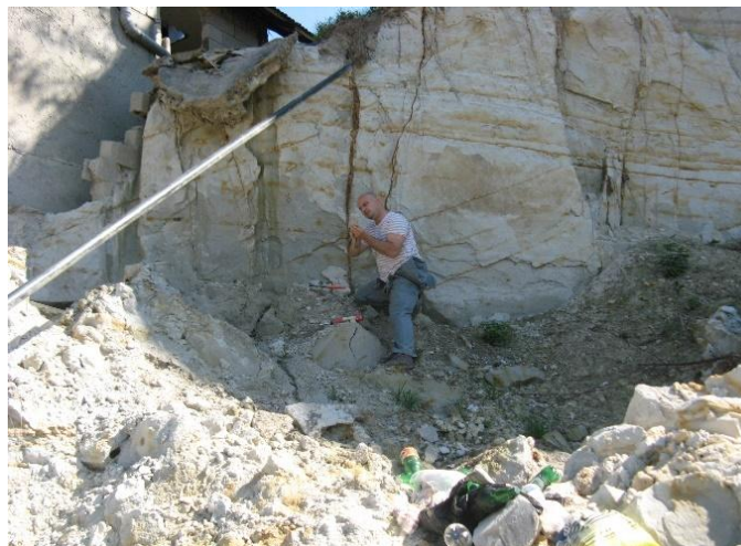
Figure 5. Measurement of crack inclination elements in the landslide scar zone. (Photo A. Čomić, 2011).
