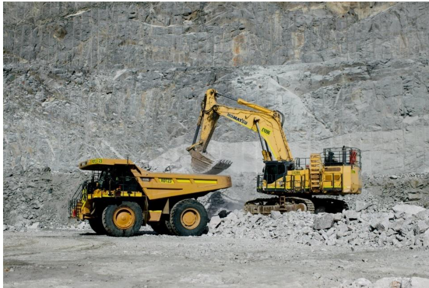
Figure 2. Lithium ore truck loading by hydraulic excavator backhoe at Talison Lithium's Greenbushes in Australia
