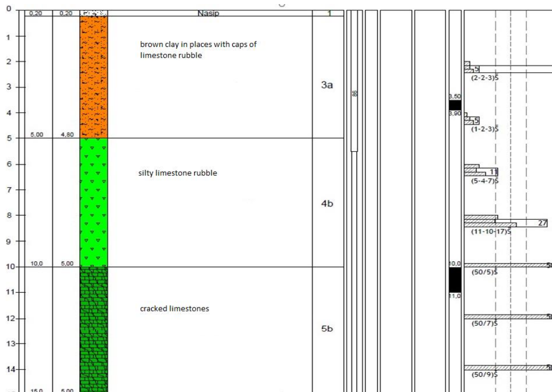
Figure 1. Lithological profile of well B - 12
