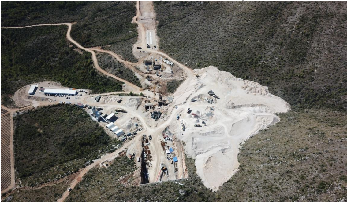
Figure 1. Location of the excavated material dump and its recycling in relation to the entrance to the tunnel [6]
