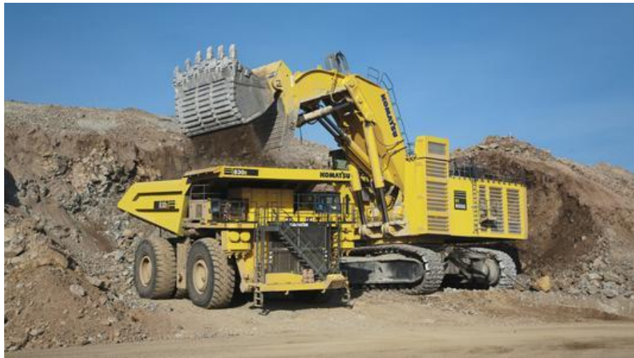
Figure 2. Loading material into a truck with a hydraulic excavator with a folding bucket
