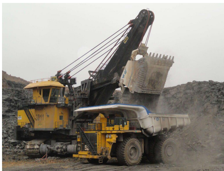
Figure 5. Loading of material with a rope shovel into a truck
