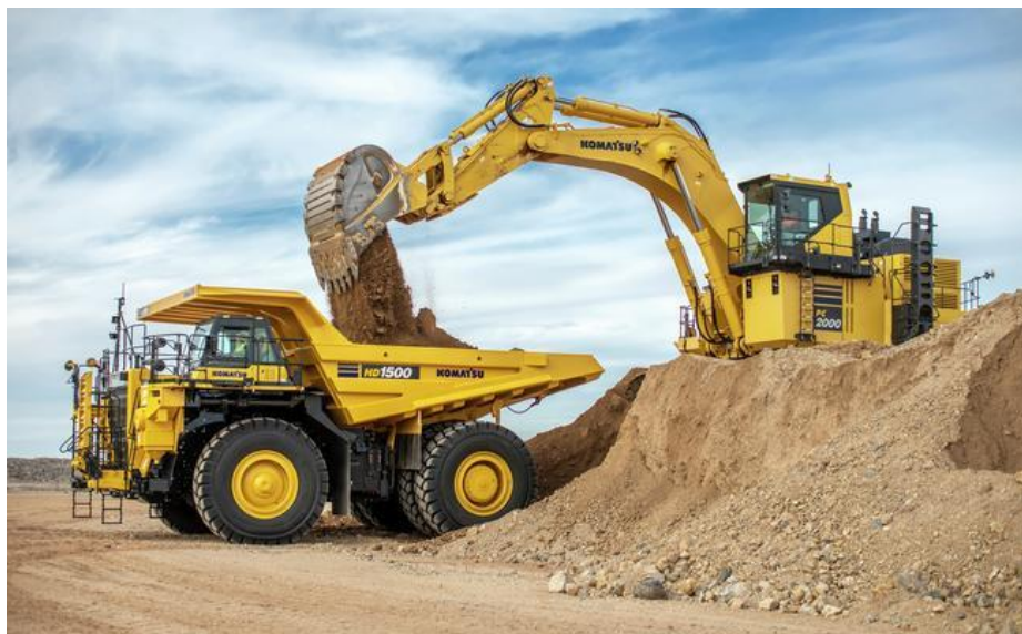
Figure 3. Loading material with a hydraulic excavator with an inverted bucket into a truck - bottom digging
