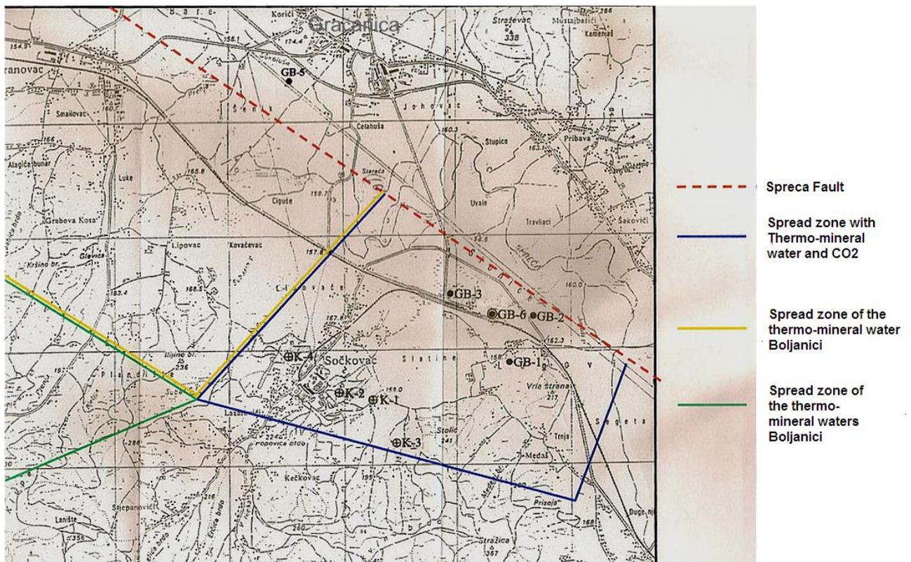
Figure 2. Spatial position of environments with different hemism of water (Scale 1 : 25000)
