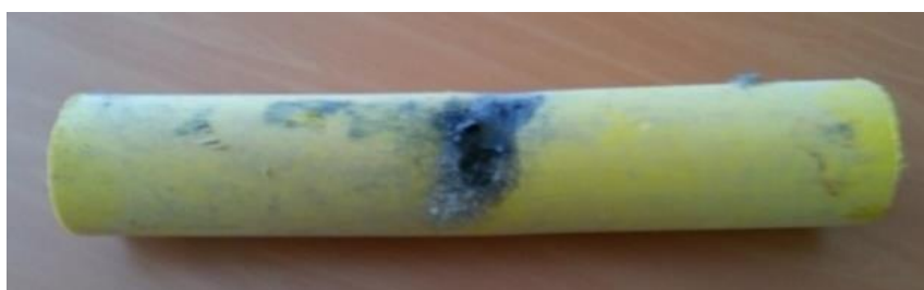
Figure 4. Damaged gas network pipe
