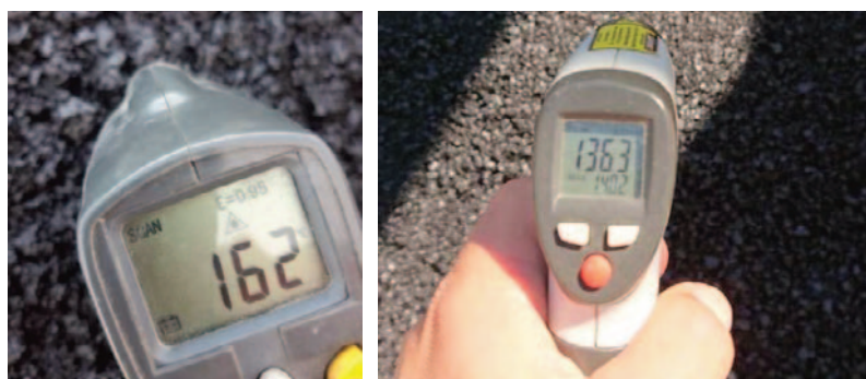
Figure 2. Production temperature and temperature during installation of asphalt at location 1 – Rastošnica; air temperature 6° C
